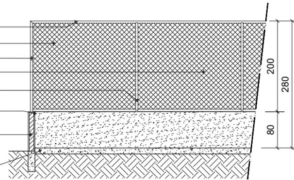
DETALHE ALAMBRADO FUNDOS - H = 2,00 m
